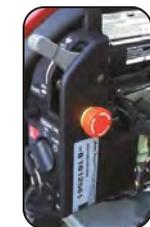
Emergency stop fitted standard on all Class B jettors
