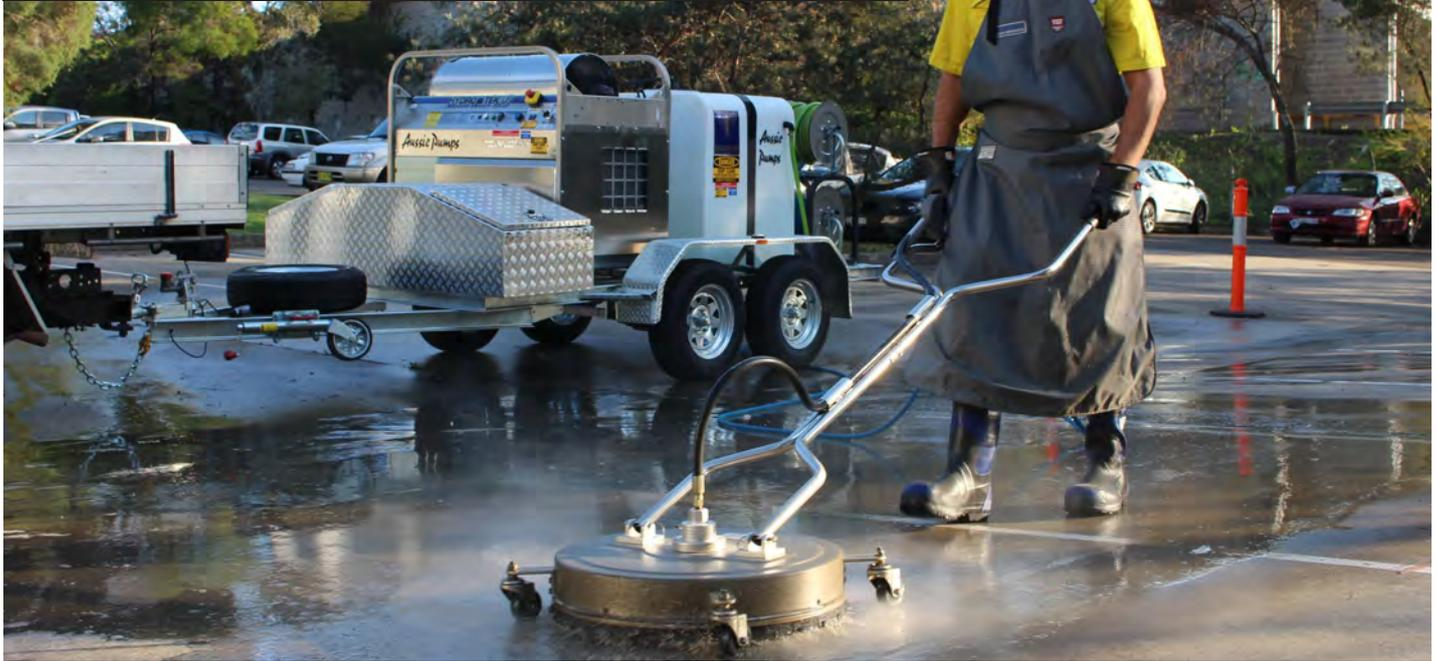
The Aussie Hydroteks are compact, high pressure, mobile steam cleaners with serious cleaning power. They are designed to perform heavy duty cleaning without needing any outside electrical power.
